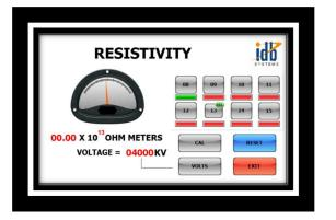
The Resistivity Meter also enables measurements to be made of charge by use of an optional screened Faraday pail and charge probe.
